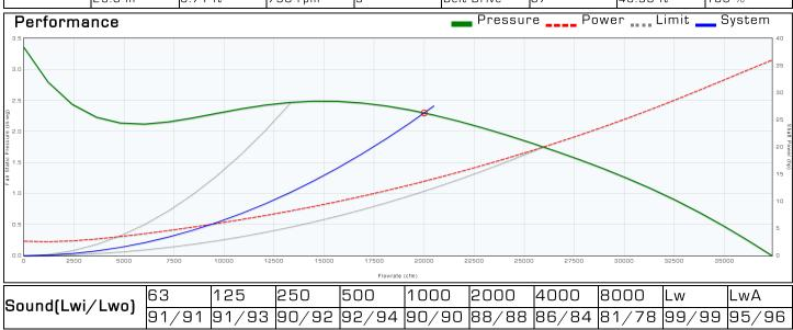
Notes: Airflow performance data are obtained in accordance with AMCA 210-07. Installed performance will vary depending on extent of cabinet geometry
