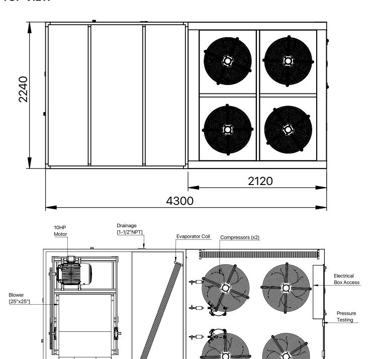
Note: All measurements are in millimeters (mm).
