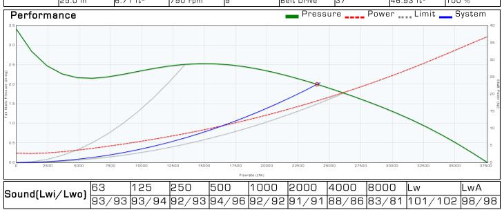
Notes: Airflow performance data are obtained in accordance with AMCA 210-07. Installed performance will vary depending on extent of cabinet geometry
